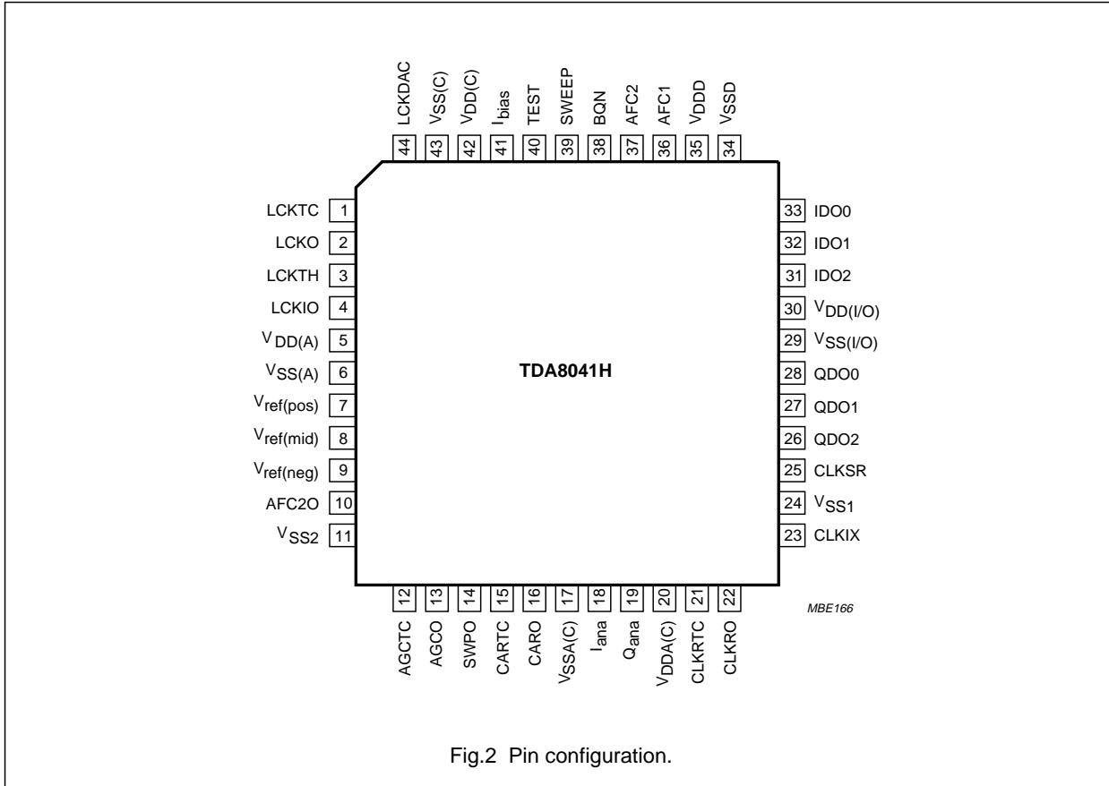
Fig.2 Pin configuration.
