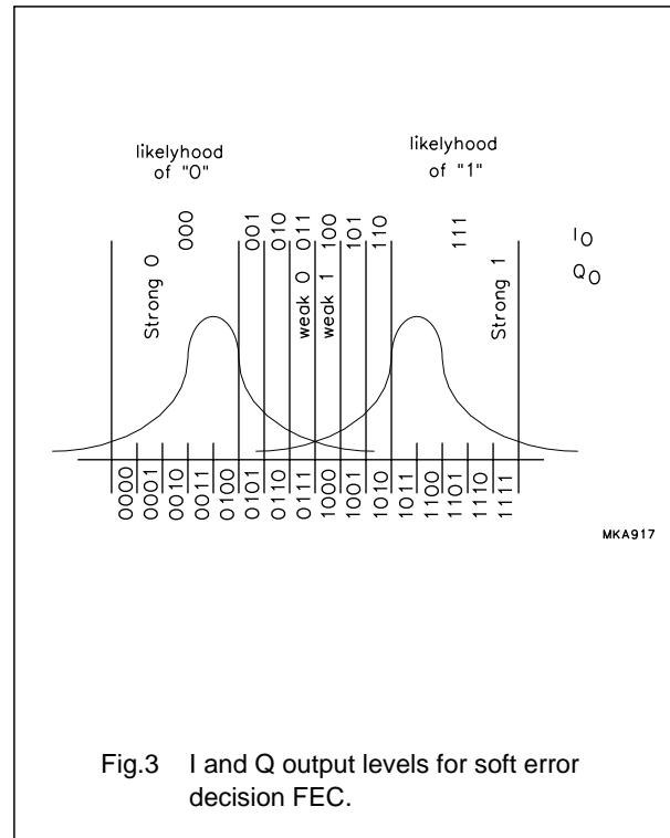
Fig.3 I and Q output levels for soft error decision FEC.
