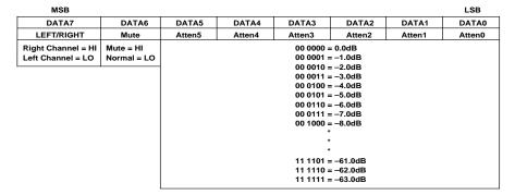
Figure 8. Serial Control Bit Definitions
