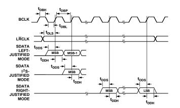
Figure 20. Serial Data Port Timing
