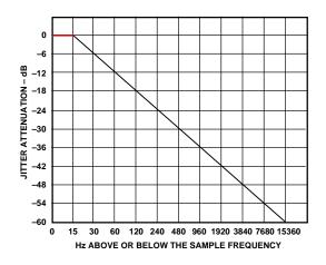
Figure 1. Digital PLL Jitter Rejection
