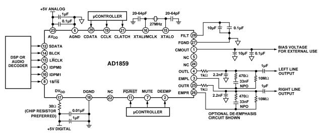
Figure 18. Recommended Circuit Connection (With De-emphasis)
