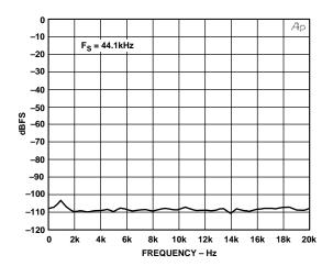
Figure 29. Channel Separation vs. Frequency at -0.5 dBFS
