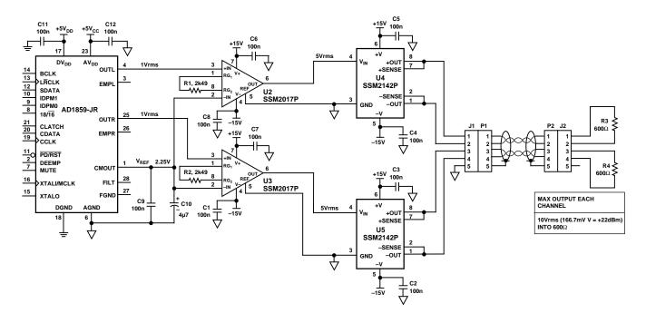
Figure 32. 600 Ohm Balanced Line Driver
