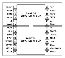
Figure 19. Recommended Ground Plane
