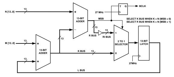
Figure 33. Numerically Controlled Oscillator Circuit
