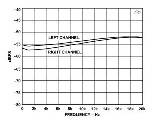
Figure 28. Power Supply Rejection to 300 mV p-p on AV<sub>DD</sub>
