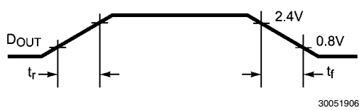
FIGURE 3. D OUT Rise and Fall Times
