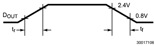
FIGURE 4. D OUT Rise and Fall Times
