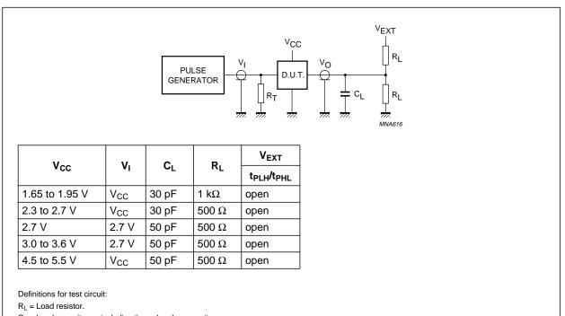
$C_L$  = Load capacitance including jig and probe capacitance.
