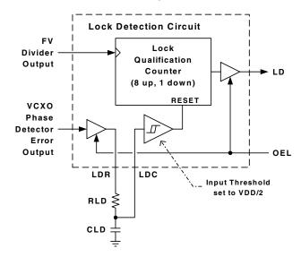
If the lock detection circuit is not used, the LDR output may remain unconnected, however the LDC input should be tied high or low. If the PCB was designed to accommodate the RLD and CLD components but the LD output will not be
