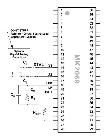
In general, the loop damping factor should be 0.7 or greater to ensure output stability. A higher damping factor will create less peaking in the passband and will further assure output stability with the presence of system and power supply noise. A damping factor of 4 will ensure a passband peak less then 0.2dB which may be required for network clock wander transfer compliance. A higher damping factor may
