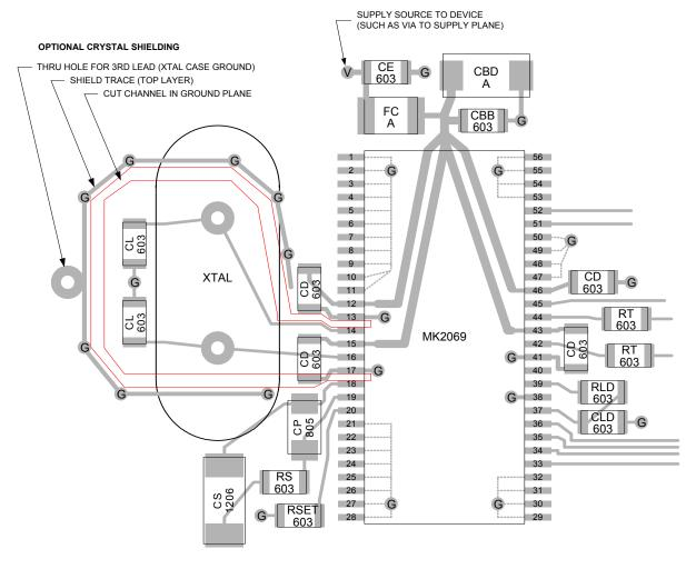
Components are identified by function (top line) and by typical package type (bottom line) which may vary.
