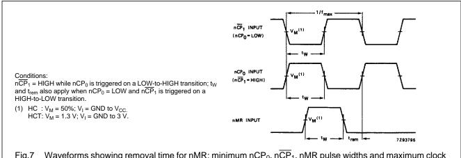
Fig.7 Waveforms showing removal time for nMR; minimum nCP<sub>0</sub>, n\overline{CP}<sub>1</sub>, nMR pulse widths and maximum clock pulse frequency.
