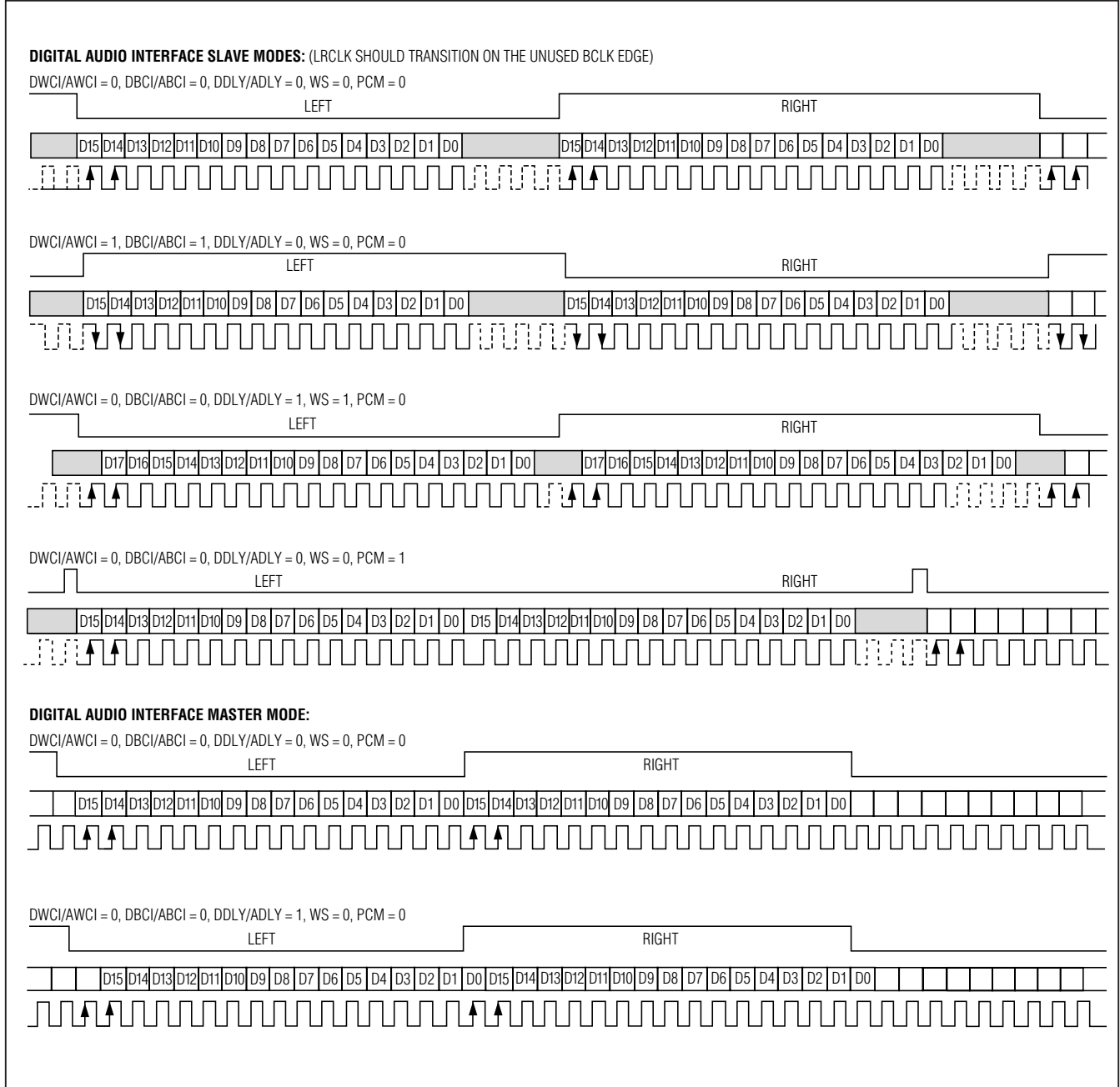
Figure 1. Digital Audio Interface Data Format Examples
