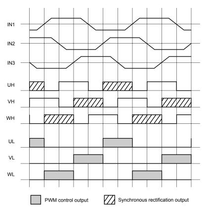
(3) When F/R = "L" and the inverting phase input as against Hall input(2).
