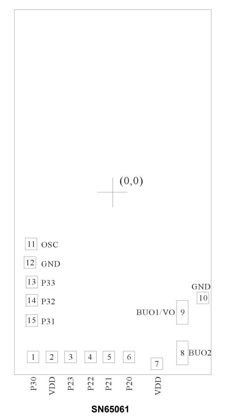
Note: The substrate MUST be connected to Vss in PCB layout.
