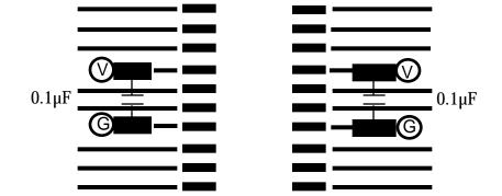
For simplicity, terminating resistors (if needed) are not shown for the outputs, but should be placed as close to the device as possible. It is most critical to have the  $0.1\mu F$  decoupling capacitors closest.
