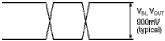
Figure 1a. Single-Ended Voltage Swing
