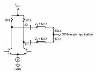
Figure 4C. CML AC-Coupled Termination
