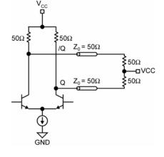
Figure 4a. CML DC-Coupled Termination
