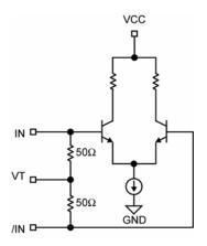
Figure 2a. Simplified Differential Input Stage
