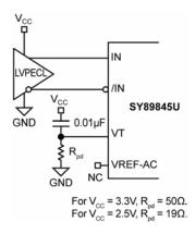
Figure 3a. LVPECL Interface (DC-Coupled)
