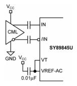
Figure 3d. CML Interface (AC-Coupled)
