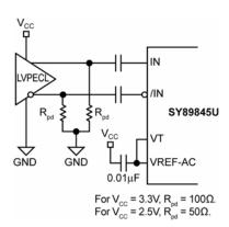
Figure 3b. LVPECL Interface (AC-Coupled)
