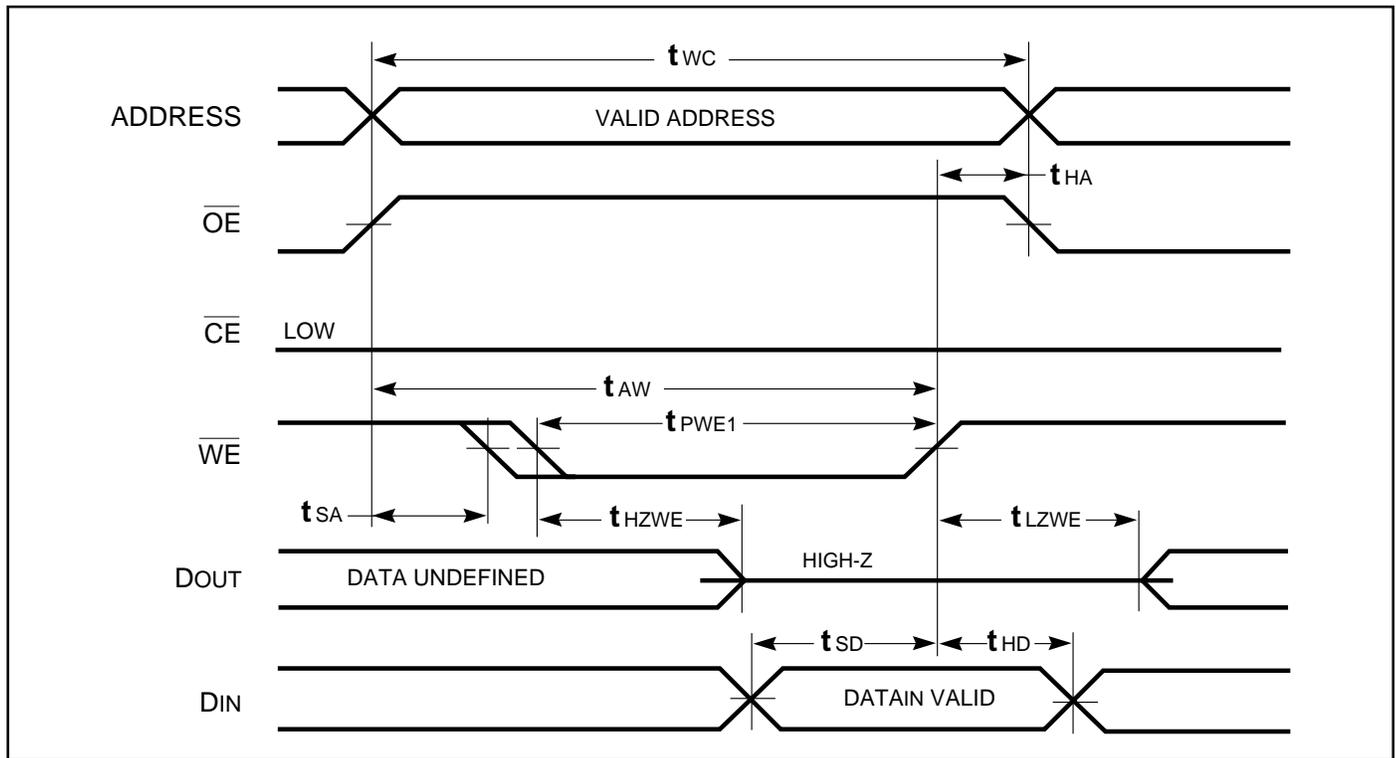
WRITE CYCLE NO. 3 ( $\overline{WE}$  Controlled,  $\overline{OE}$  is LOW During Write Cycle) <sup>(1)</sup>
