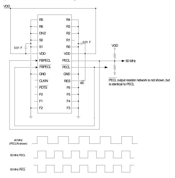
Note: The series termination resistor is located before the feedback
