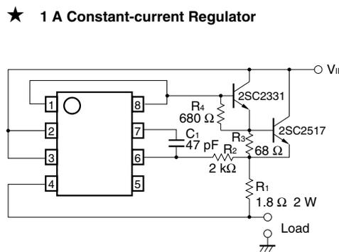
**Caution** Note the power consumption of the  $\mu$  PC305 when the output pin is short-circuited and that of the external transistor.
