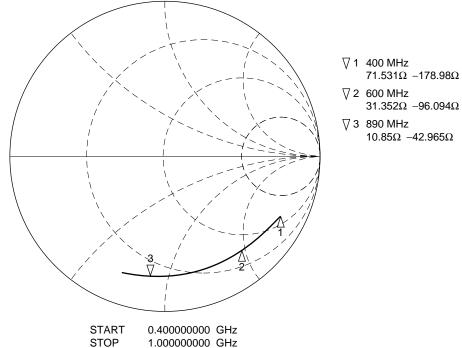
**OUTPUT IMPEDANCE (by measurement circuit 5)**
