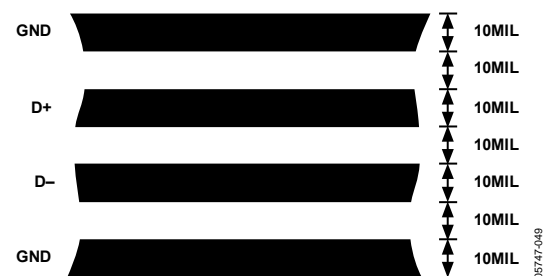
Figure 37. Arrangement of Signal Tracks
