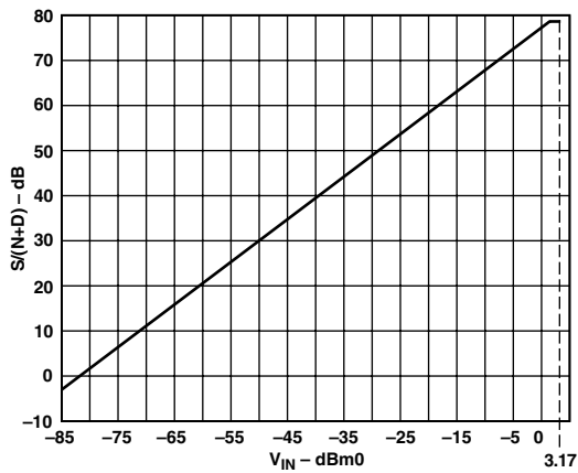
Figure 5a. S/(N+D) vs. V_{IN} (ADC @ 3 V) over Voiceband Bandwidth (300 Hz – 3.4 kHz)
