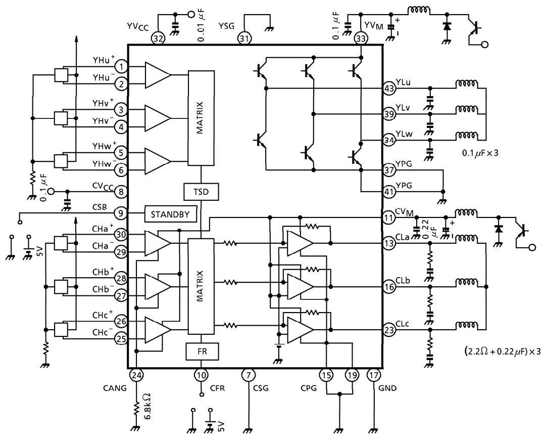
(Note) Utmost care is necessary in the design of the output line, YVM, CVM and GND line since IC may be destroyed due to short-circuit between outputs, air contamination fault, or fault by improper grounding.
