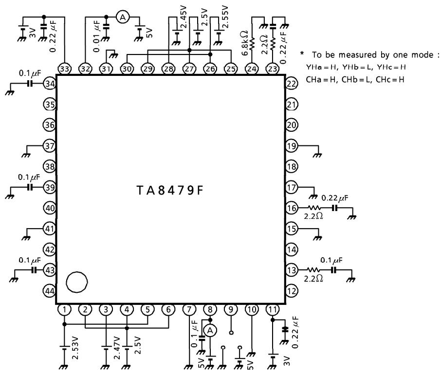
2. YM<sub>M</sub>, CM<sub>M1</sub>, CM<sub>M2</sub>
