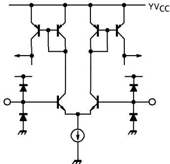
The Hall amp is a differential amp, and the common-phase input voltage range is  $YV_{CMR} = 1.3 \sim YV_{CC} - 1.3$  [V]. For signals from Hall elements, input sinusoidal waves. Noise, etc., which causes malfunction when found in signals, must be prevented by a condenser.
