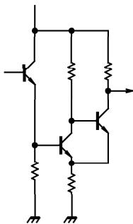
When the temperature exceeds  $T_j = 170^\circ\text{C}$  (Typ.) (design target value), the output circuits in the capstan and cylinder sections are turned off. This circuit has an approximately  $30^\circ\text{C}$  Hysteresis, and the recovery temperature is  $T_j = 140^\circ\text{C}$  (Typ.) (design target value).
