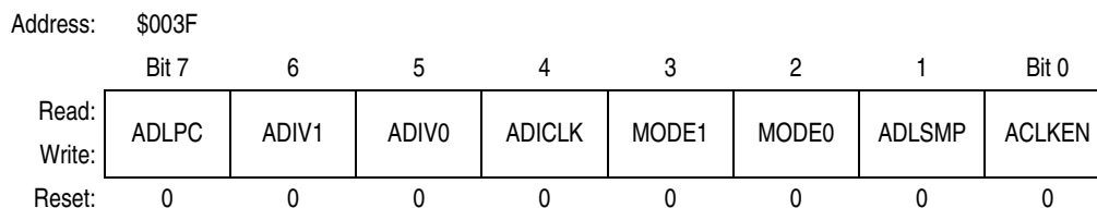
Figure 3-7. ADC10 Clock Register (ADCLK)
