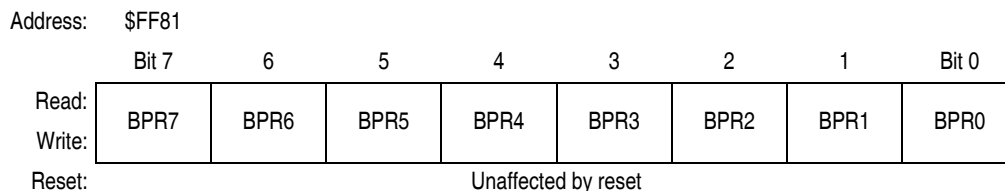
Figure 2-8. FLASH-2 Block Protect Register (FL2BPR)
