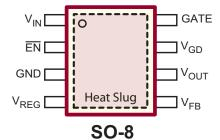
Backside on the SO-8 package is at ground potential and may be connected to ground or left unconnected.
