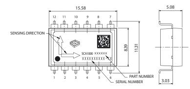
Acceleration in the direction of the arrow will increase the output voltage.
