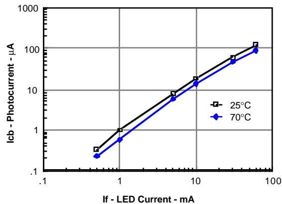
**Figure 8. Base current versus If and HFE**
