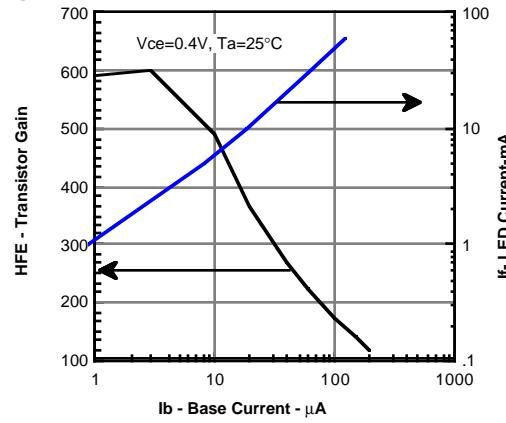
**Figure 9. Normalized HFE versus Ib, Ta**
