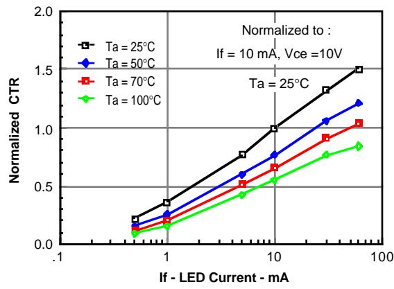
**Figure 5. Normalized saturated CTR**
