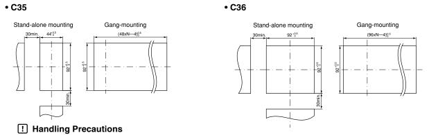
• When three or more units are gang-mounted horizontally, the maximum allowable ambient temperature is 40°C.
