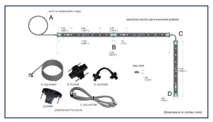
Total power consumption of modules should not exceed rating of power supply
