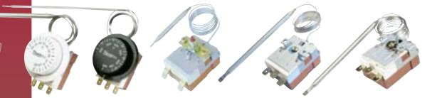
Thermtrol offers the versatile TS Series of adjustable bulb and capillary thermostats suitable for applications requiring variable temperature setting ability and remote control. The TS Series design incorporates a changeover thermal switch and an auxiliary switch useful for fan control or alarm signal. A variety of available features, a large in-stock inventory, and a surprisingly low price combine to make the Thermtrol TS Series an excellent value.
