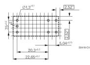
$^{\ast})$  With the recommended PCB hole sizes a grid pattern from 2.5 mm to 2.54 mm can be used.
