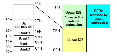
MG87FE/L04 has internal data RAM that is mapped into three separate segments. They are lower 128 bytes of RAM, upper 128 bytes of RAM and 128 bytes Special Function Register (SFR).
