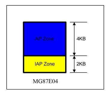
In MG87FE/L04, the first partition named AP-memory is the space for storing user's application program code. The second one named as IAP-memory and the space which is accessed by CPU for storing the user data. The third is named as ISP-memory and it is special for ISP boot code program.
