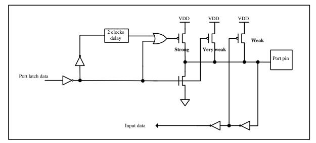
By the way, the pull-up resistor is disabled on P10/P11 in default.
