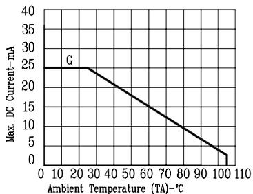
Fig5. MAX. ALLOWABLE DC CURRENT VS. AMBIENT TEMPERATURE.
