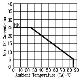
Fig5. MAX. ALLOWABLE DC CURRENT VS. AMBIENT TEMPERATURE.
