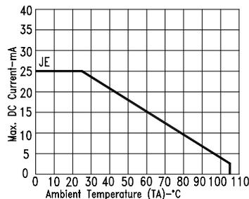
Fig5. MAX. ALLOWABLE DC CURRENT VS. AMBIENT TEMPERATURE.
