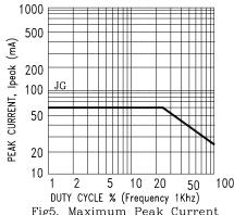
Fig5. Maximum Peak Current vs. Duty Cycle %
