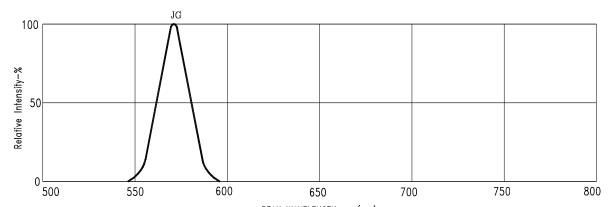
PEAK WAVELENGTH p (nm) Fig1.Spectral Emission
