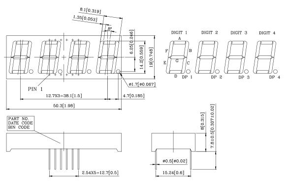
NOTES: 1.All dimensions are in millimeters. Tolerances are ± 0.25 mm (0.01") unless otherwise noted.
