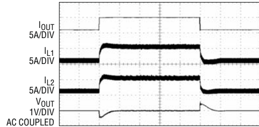
V_{IN} = 24V V_{OUT} = 48V \Delta I_{OUT} = 1A \text{ TO } 5A
