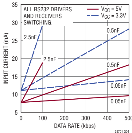
V_{CC} Supply Current vs RS232 Data Rate
