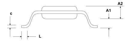
28-Pin SSOP Package Dimensions
