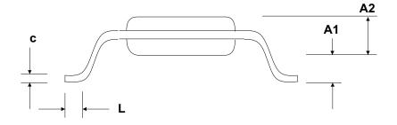
28-Pin SSOP Package Dimensions
