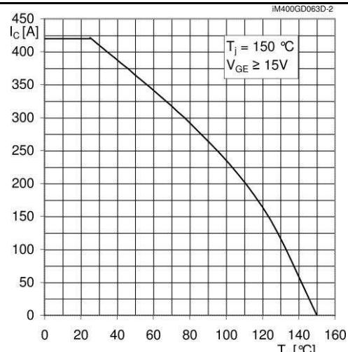
Fig. 2 Rated current vs. temperature  $I_C = f(T_s)$
