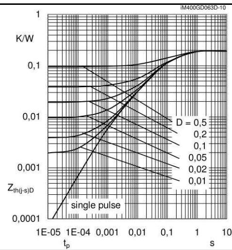
Fig. 10 Transient thermal impedance of FWD
