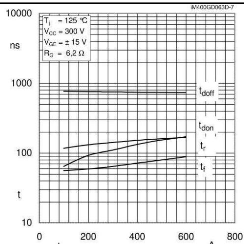
Fig. 7 Switching times vs.  $I_c$
