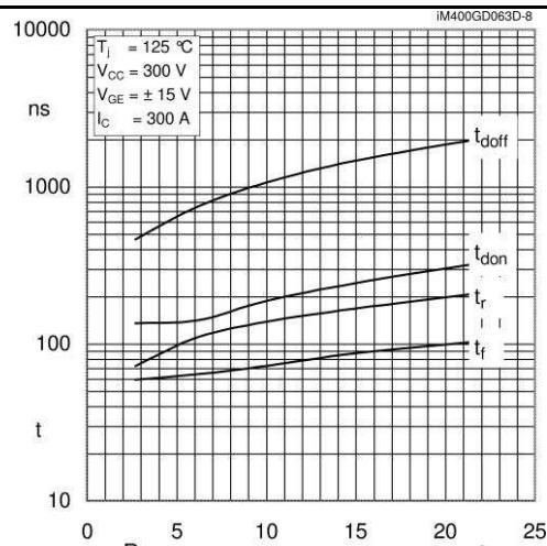
Fig. 8 Switching times vs. gate resistor  $R_G$
