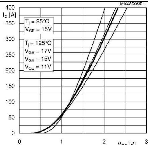
Fig. 1 Output characteristic, inclusive  $R_{CC} + EE'$
