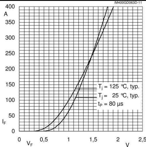
Fig. 11 CAL diode forward characteristic, incl.  $R_{CC' + EE'}$
