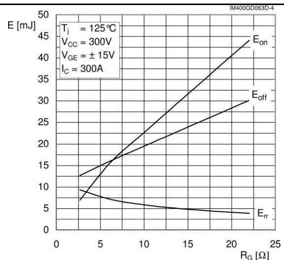
Fig. 4 Turn-on /-off energy =  $f(R_G)$
