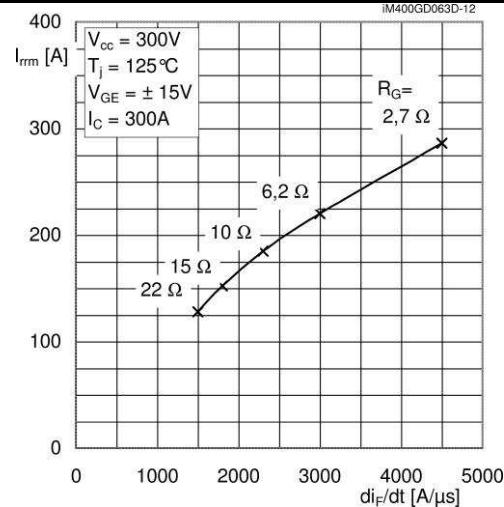
Fig. 12 CAL diode peak reverse recovery current
