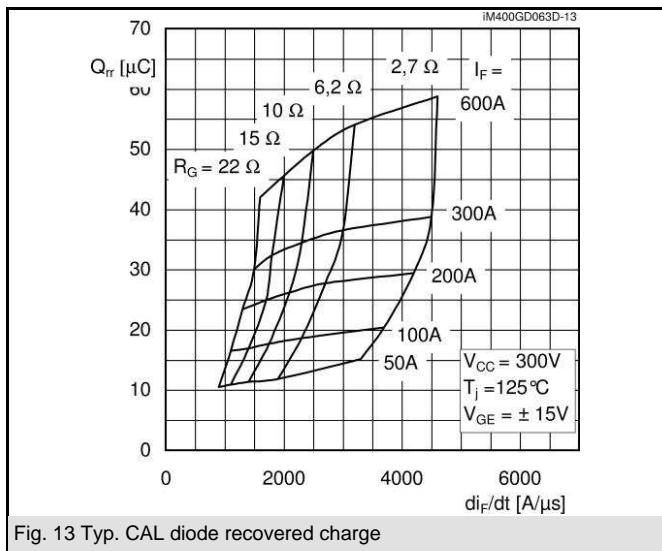
Fig. 13 Typ. CAL diode recovered charge
