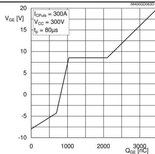
Fig. 6 Gate charge characteristic
