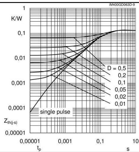
Fig. 9 Transient thermal impedance of IGBT
