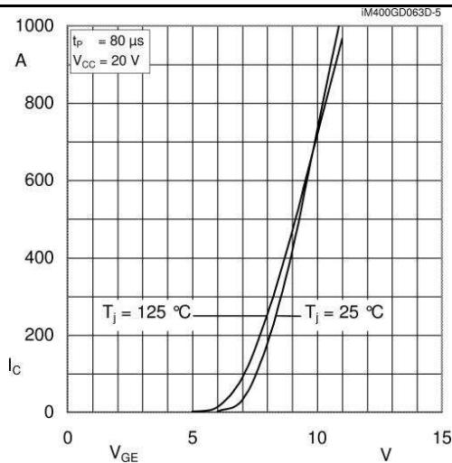
Fig. 5 Transfer characteristic
