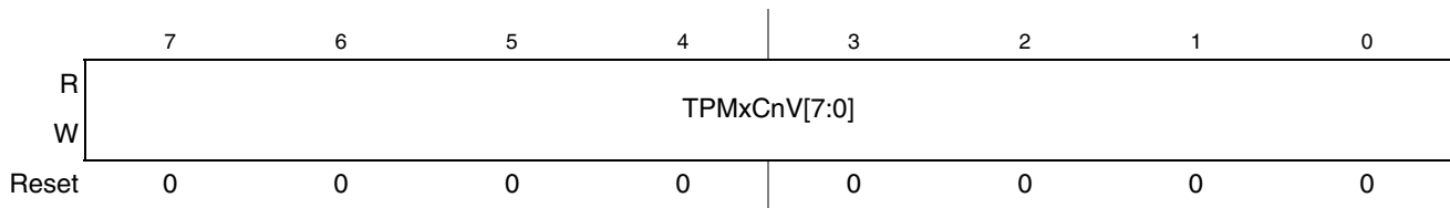
Figure 21-13. TPM Channel Value Register Low (TPMxCnVL)
