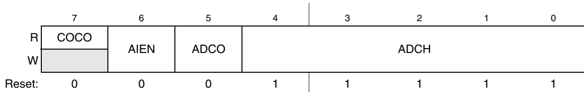
Figure 9-2. Status and Control Register (ADCSC1)
