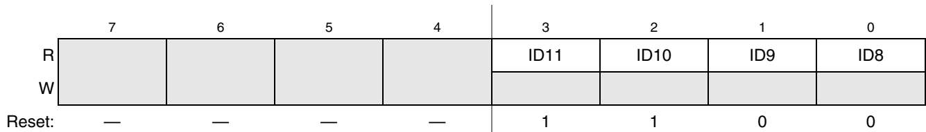
Figure 5-5. System Device Identification Register — High (SDIDH)
