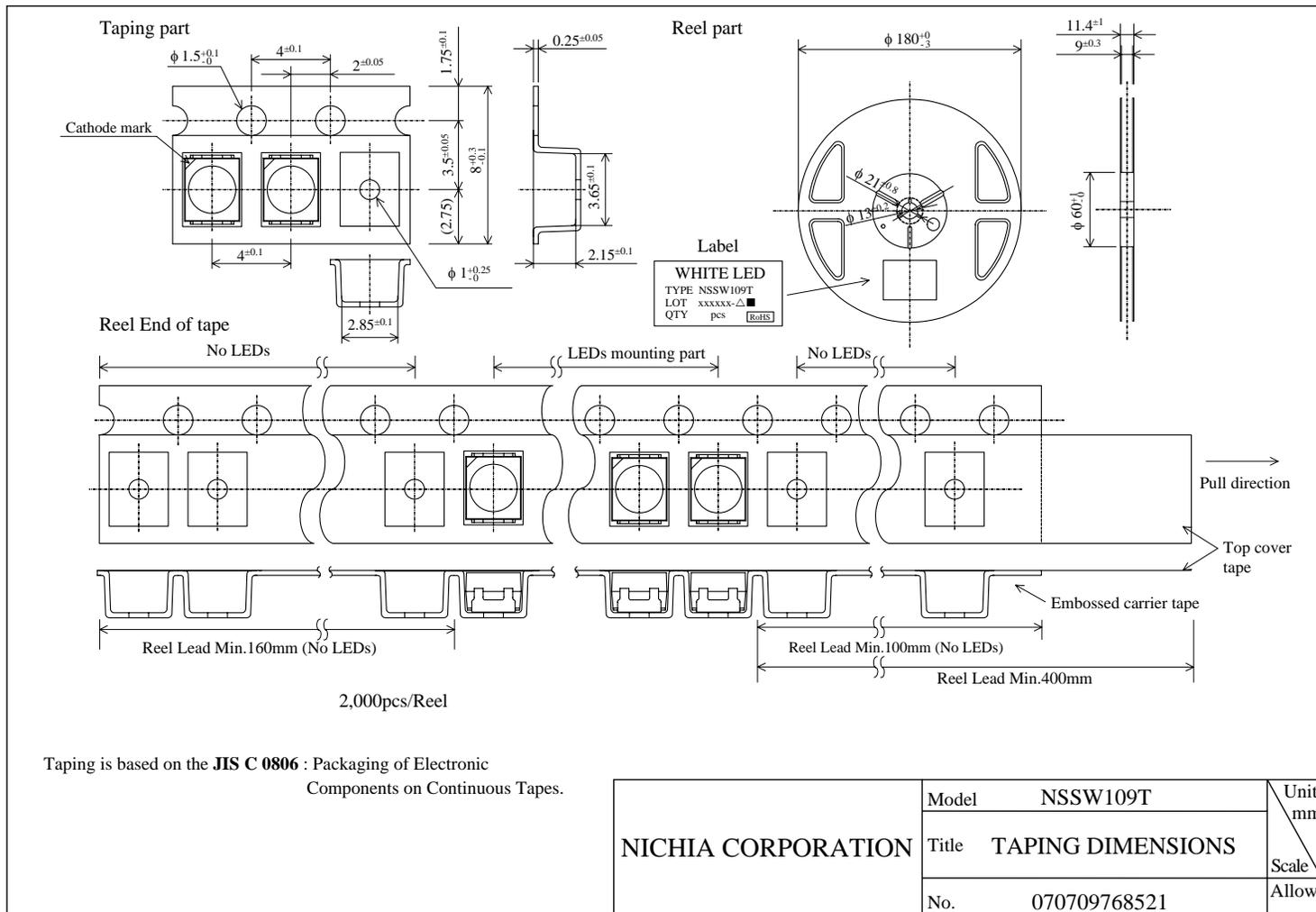
Taping is based on the **JIS C 0806** : Packaging of Electronic Components on Continuous Tapes.
