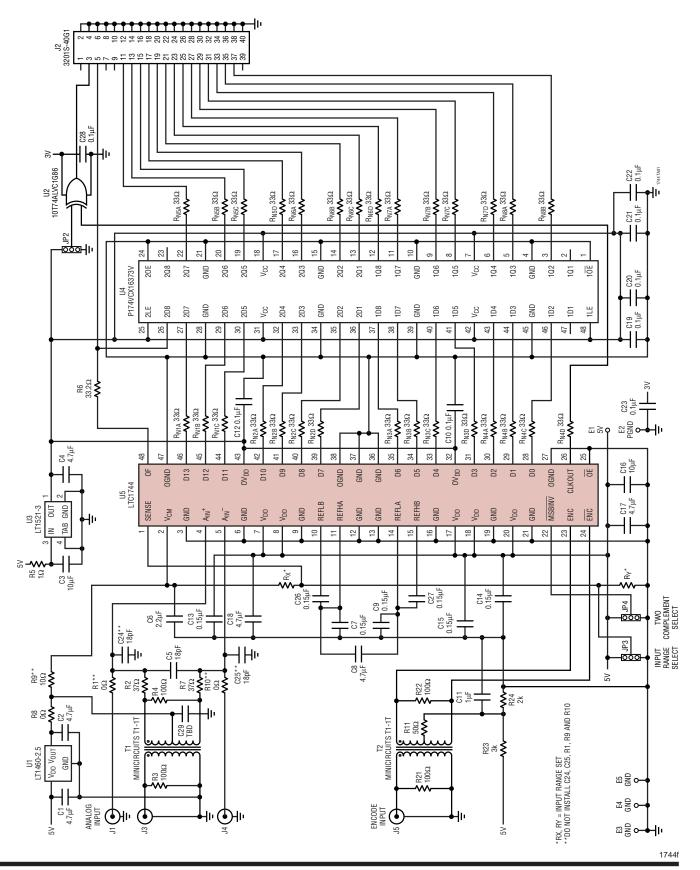
DC345B Evaluation Circuit Schematic of the LTC1744
