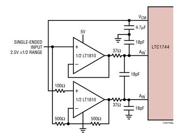
Figure 4a. Differential Drive with Op Amps
