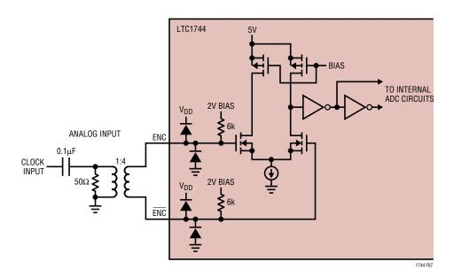
Figure 7. Transformer Driven ENC/ENC
