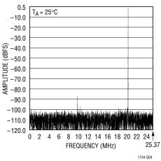
Nonaveraged, 8192 Point FFT, Input Frequency = 2.5MHz, -1dB, 3.2V Range
