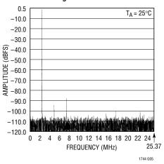
Nonaveraged, 8192 Point FFT, Input Frequency = 20MHz, -1dB, 3.2V Range
