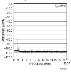
Averaged, 8192 Point FFT, Input Frequency = 51MHz, -6dB, 2V Range
