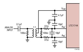
Figure 3. Single-Ended to Differential Conversion Using a Transformer
