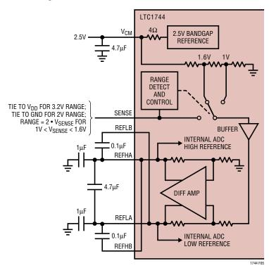
Figure 5. Equivalent Reference Circuit
