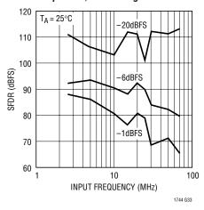
SFDR vs Input Frequency and Amplitude, 2V Range
