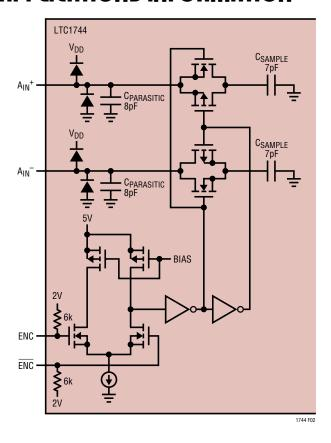
Figure 2. Equivalent Input Circuit
