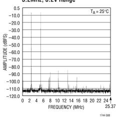
Averaged, 8192 Point FFT, Input Frequency = 2.5MHz, -6dB, 2V Range
