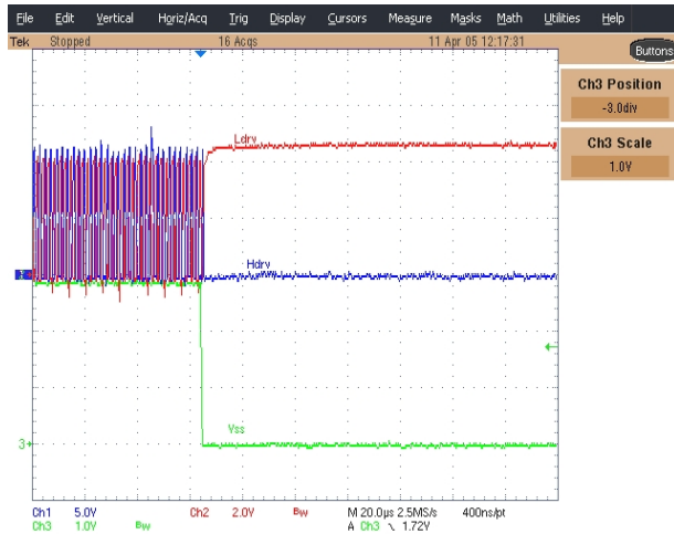
Figure 18 - Shutdown by shorting the SS pin Ch1: Hdrv, Ch2: Ldrv, Ch3:SS I Load =5A
