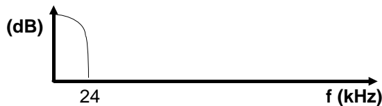
Figure 26. Spectrum After Continuous Time Filter
