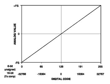
Figure 22. Linear Transfer Functions
