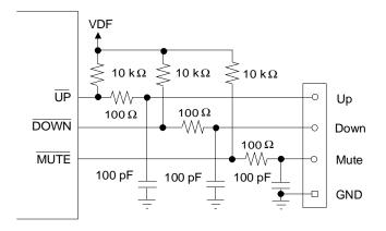
Figure 24. Volume Control Circuit
