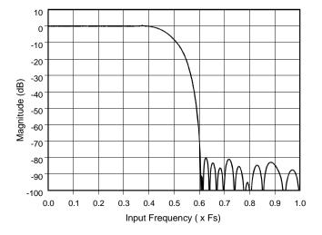
Figure 34. ADC Filter Response
