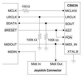
Figure 13. CS9236 Wavetable Serial Port Interface
