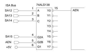
Figure 2. 16-bit Decode Circuit
