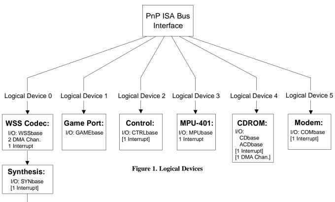
Logical Device 5 supports a modem connected to the peripheral port. This interface, on the external peripheral port, supports modems with 2 to 256 I/O locations (only SA2-SA0 are buffered through the part) and supports a base address and an interrupt. Although this logical device is listed as a modem, any external device that fits within the resources listed above may be substituted.
