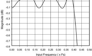
Figure 35. ADC Passband Ripple
