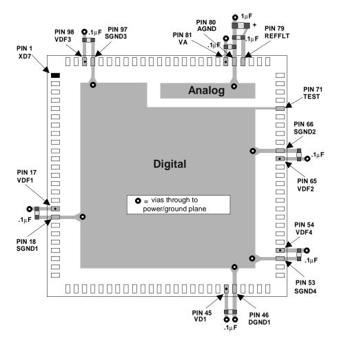
Figure 33. Recommended Decoupling Capacitor Positions
