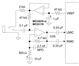
Figure 28. Left or Mono Microphone Input
