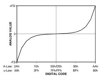
Figure 23. Companded Transfer Functions
