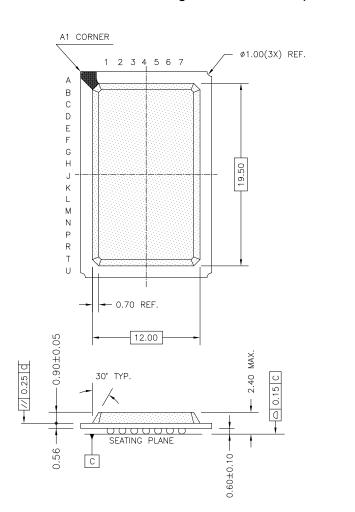
Figure 2. 119-ball BGA (14 × 22 × 2.4 mm), 51-85115
