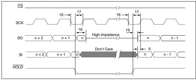
FIGURE 1-2: SERIAL INPUT TIMING
