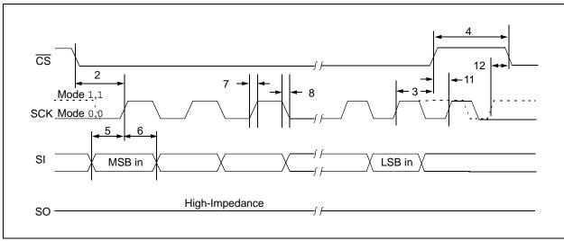
FIGURE 1-3: SERIAL OUTPUT TIMING
