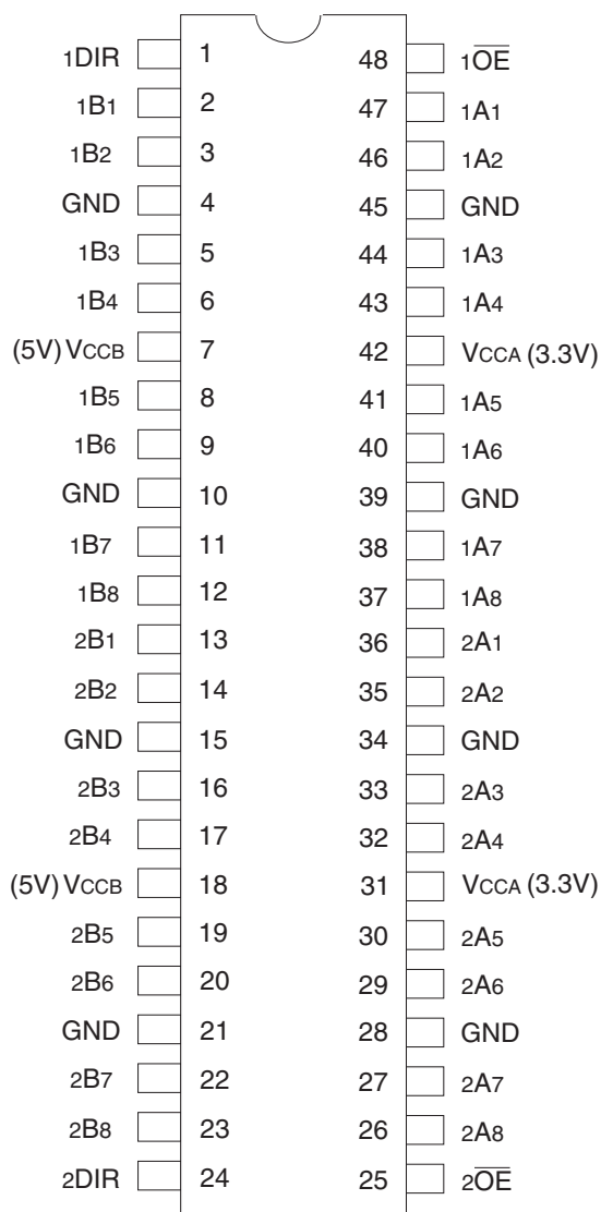
SSOP/ TSSOP TOP VIEW
