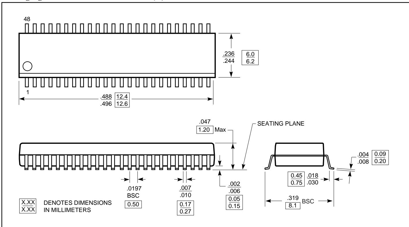
**Packaging Mechanical: 48-Pin SSOP (V)**
